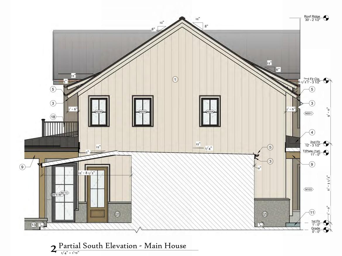
ALL NEW WINDOWS TO BE MARVIN ULTIMATE SERIES WITH SDLS AND BLACK SPACER BARS. ALL GLAZING SHALL BE CLEAR INSULATED GLASS WITH VERIFY ALL ROUGH OPENING SIZES WITH SELECTED WINDOW VENDOR PRIOR TO FRAMING
